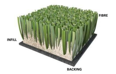
The structure of the artificial turf surface has three basic elements:
