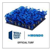
Latest generation artificial turf, manufactured with the TUFTING system. It has a gauge of 3/16" with 22 tufts/dm, resulting in 46.200 tufts/m². The Supercourt XN available in different colors turf filament has a height of 10 mm and 10.000 dtex.
